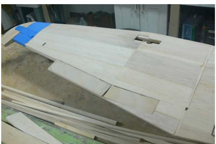
Stabilizer and elevator construction. The prototype had fabric covered tail surfaces, but I will cover them with 1/16" balsa.
